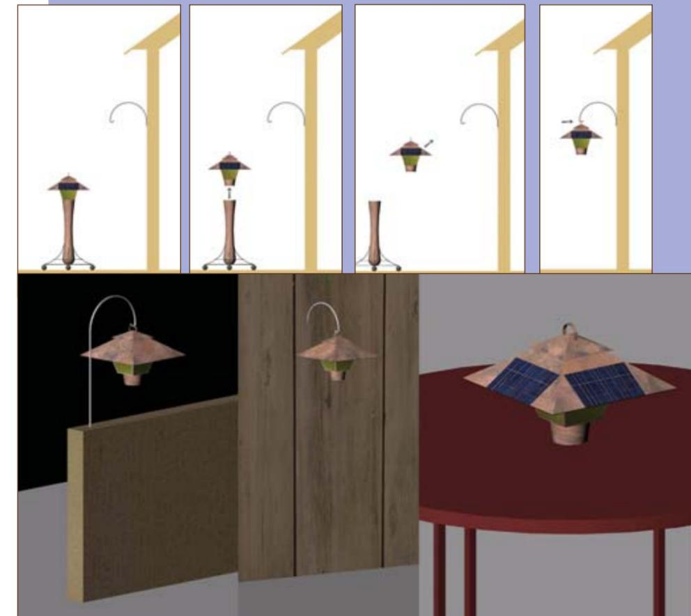
(Figure 5) Versatility of portable bollard; arm-mounted on parking area wall (left), on courtyard wall or outside garages (center), and with canopy removed from base to act as lantern on table top (right).
