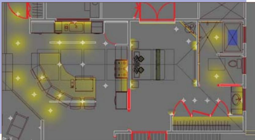
(Figure 7) Plan view of kitchen area on the left and master bedroom on the right, with lighting zones highlighted in yellow.
