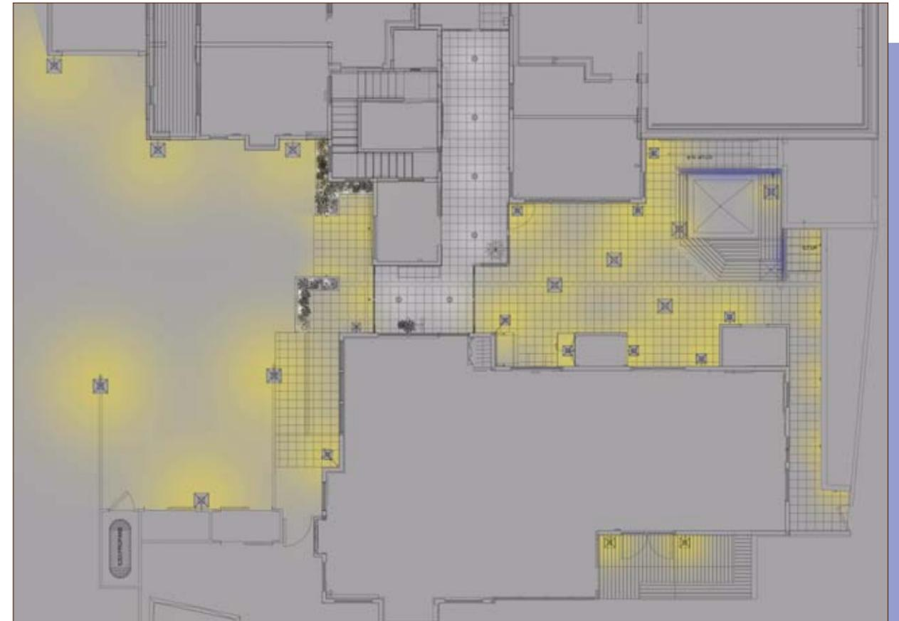
(Figure 1) Plan view showing soft exterior lighting from the front parking area, plant beds (left), and garages through the entrance and vestibule to the rear courtyard, where color-changing LEDs illuminate the glass block walls flanking the hot tub. All lighting projects downward, respecting The Sea Ranch zero-light pollution policy.
